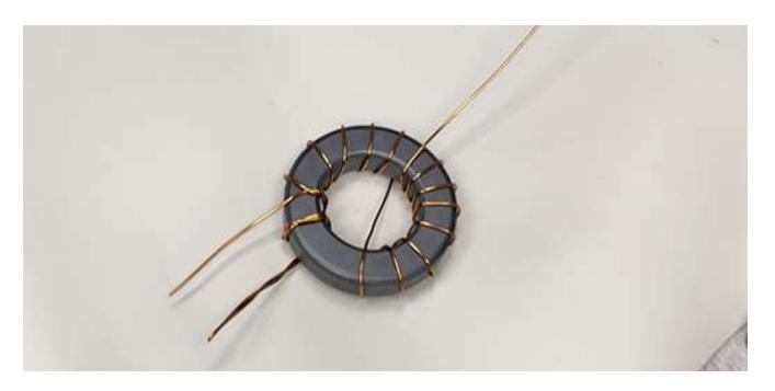
Find the point where the two pieces of wire become one, and place this on the toroid. Wrap the double part twice around the core. Then wrap the other 12 windings as shown, crossing the wire over to the other side of the toroid after the sixth wind.
