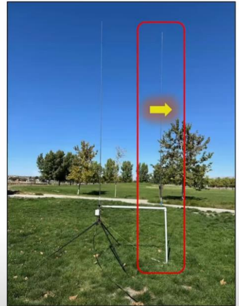
Dominator 2-Element Vertical Beam for 10M pointed east at US-3473 in California. Parasitic director creates up to +4 dB gain across four bands: 17M-10M.
